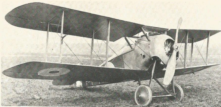
Based on the Snipe, which it resembled externally, the Salamander was a trench fighter with 650 lb. of armour protection for the nose section. Over 183 Salamanders were built
