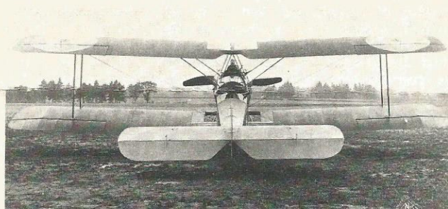
Above: South to North view of a 1 1/2 Strutter showing the centre-section strut arrangement from which the aircraft got its name, the open section of the lower wing roots, the single forward-firing Vickers gun and the Scarff ring for the Lewis gun. Over 5,400 1 1/2 Strutters were built (about 4,200 of them in France) and one specimen is still preserved in the Brussels Military Museum
