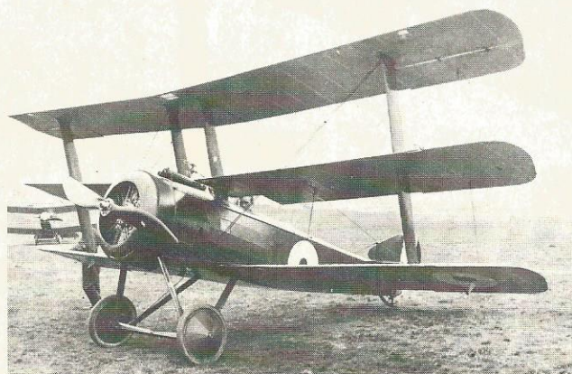
Below: Sopwith Triplane single-seat fighter powered by a 110-h.p. Clerget engine (although some had the 130-h.p. Clerget). It was the first triplane to enter service in W.W.I and 152 were built—103 by Sopwith's at Kingston, 46 by Clayton and Shuttleworth, and 3 by Oakley
